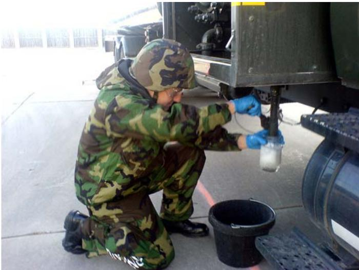
**Staff Sgt. Joel Noell from the 507<sup>th</sup> Mission Support Groups Logistics Readiness Squadron's Petroleum, Oil and Lubricant (POL) section draws a sample from a fuel truck to conduct a visual examination.**
