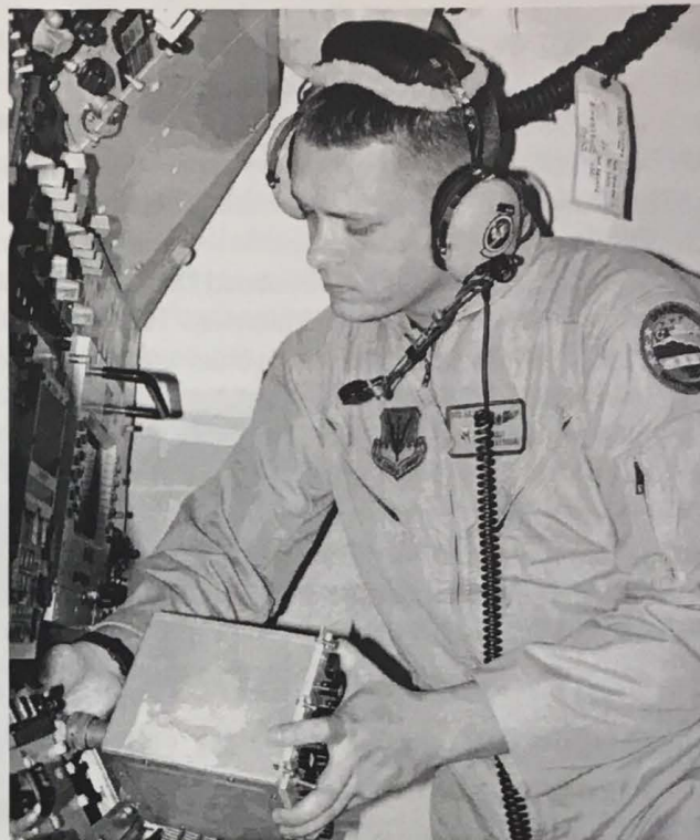
SSgt. Shawn Kilbourne, 970 th Expeditionary Airborne Air Control Squadron communications technician, replaces a mission audio panel Oct. 1 during an ONW mission.
