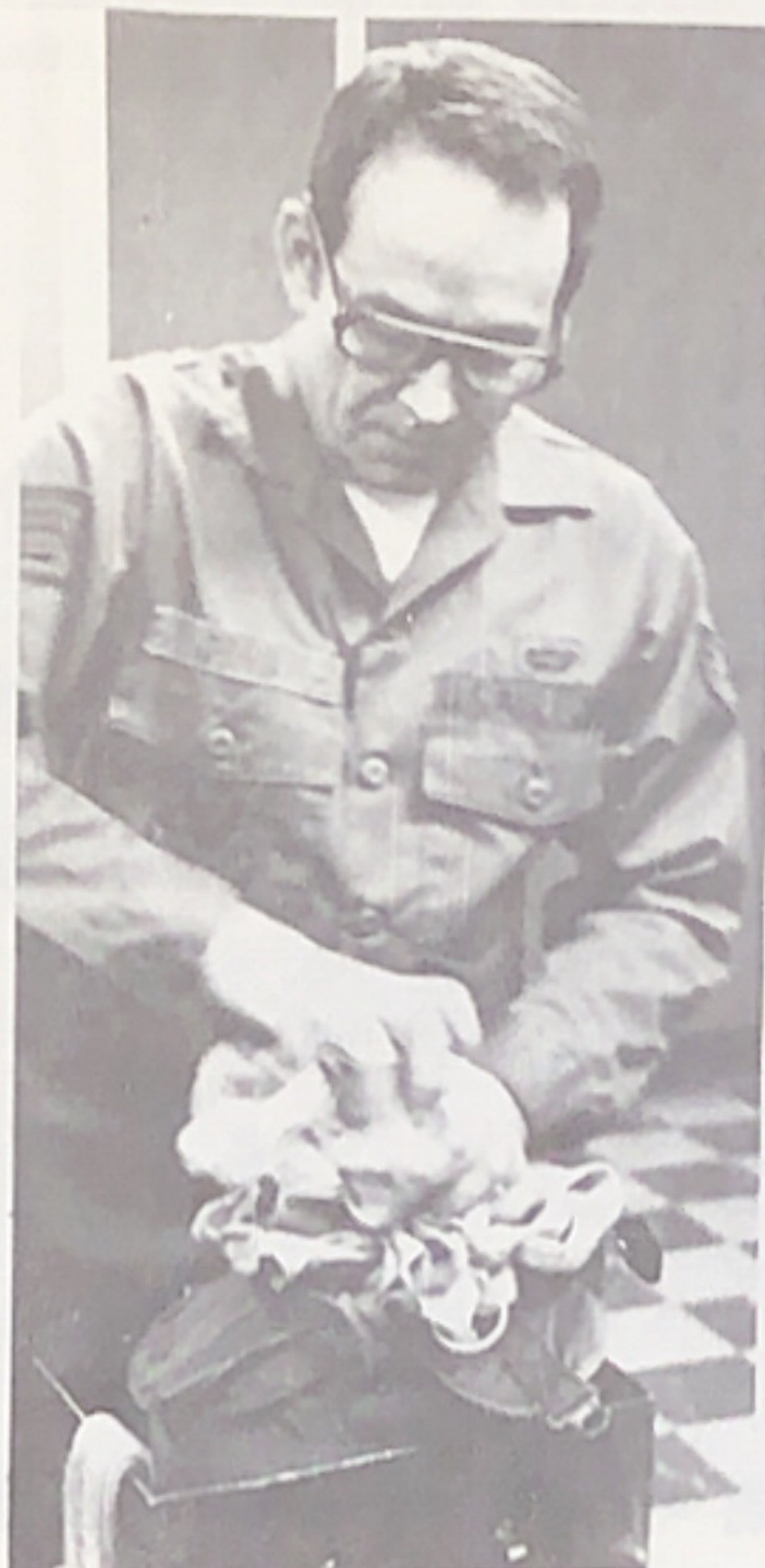
SSgt Ford compressing the pilot chute spring, the final step in packing a drag chute.
