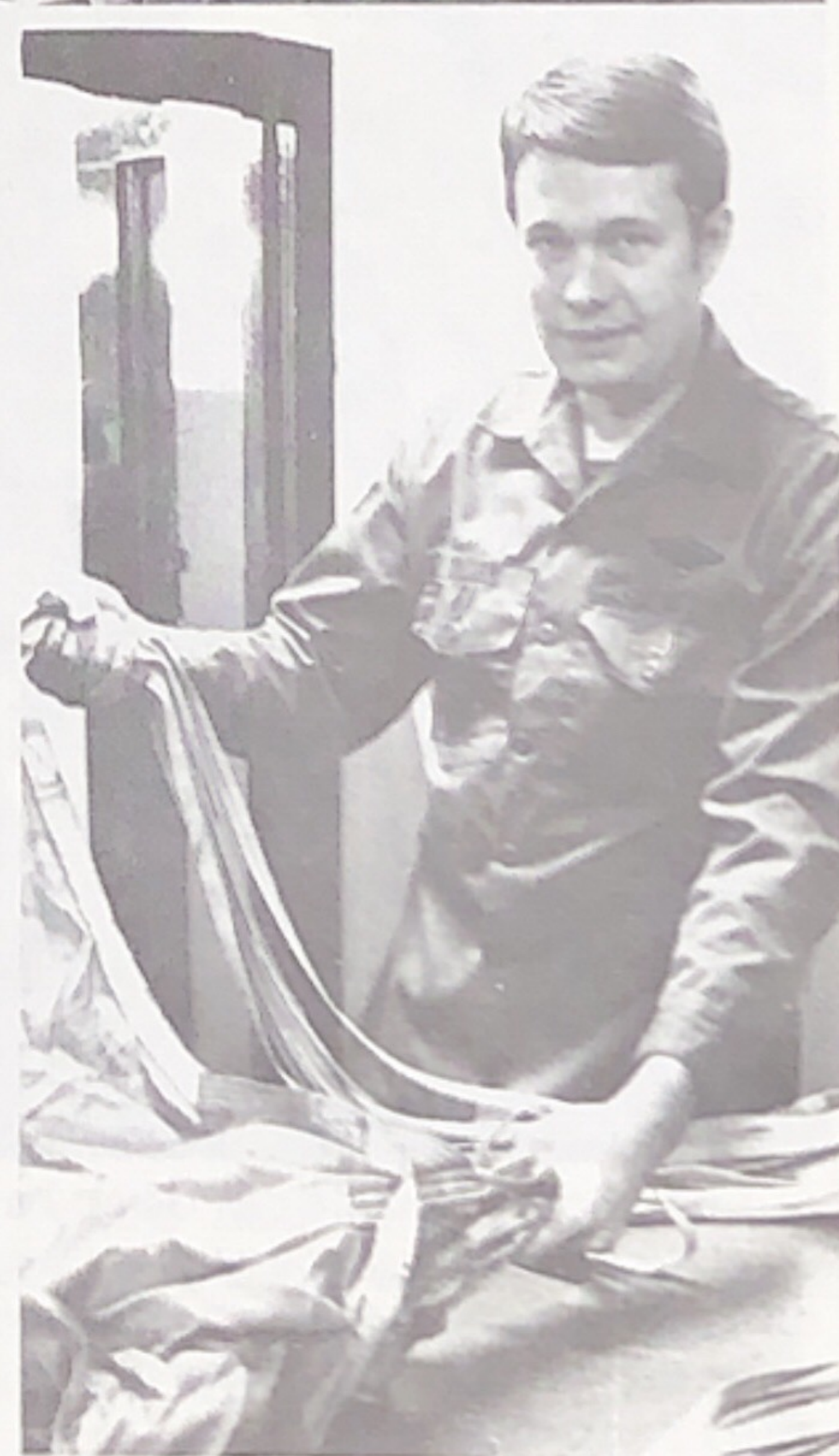
Sgt collier seperating the shroud lines and folding the canopy prior to packing a drag chute. (USAF photos)
