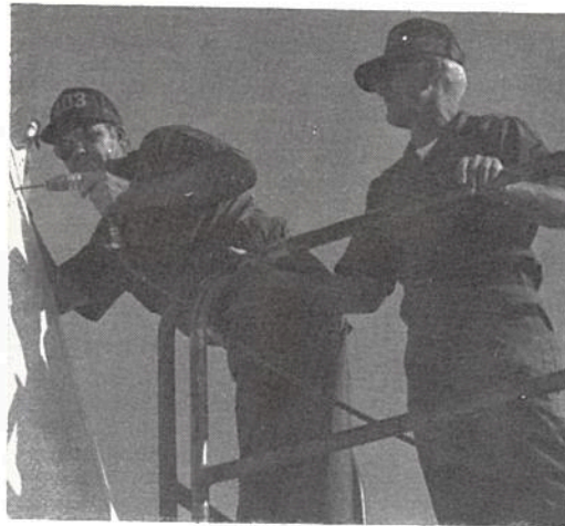
SMSgt's Wessley Winters and Darrell Lumry of the 403rd CLSS restore a C-47 Skytrain for display at Tinker AFB. The project involved removal of heater inlets and exhausts, antenna masts, and rotating beacon lights and patching the holes. (USAF photo)
