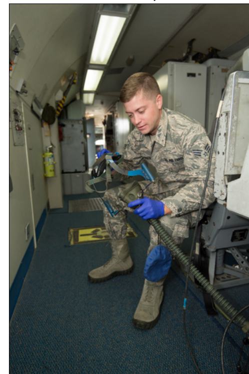
Senior Airman Chris Ogden, an aircrew flight equipment specialist from the 513th Operations Support Squadron, inspects an oxygen mask on board an E-3 Sentry.
