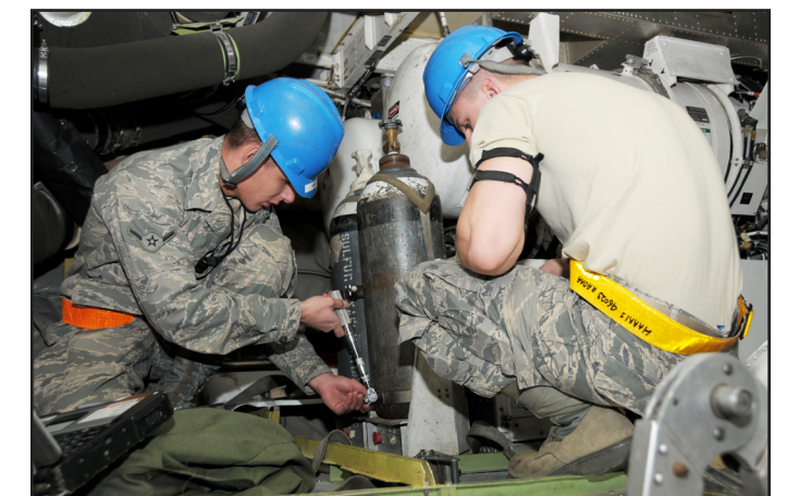
Airman Robert Duncan and another maintainer of the 513 MXS work on a support system for the AWACS radar during the LCAP inspection last UTA. (U.S. Air Force Photo//SrA Caleb Wanzer)
